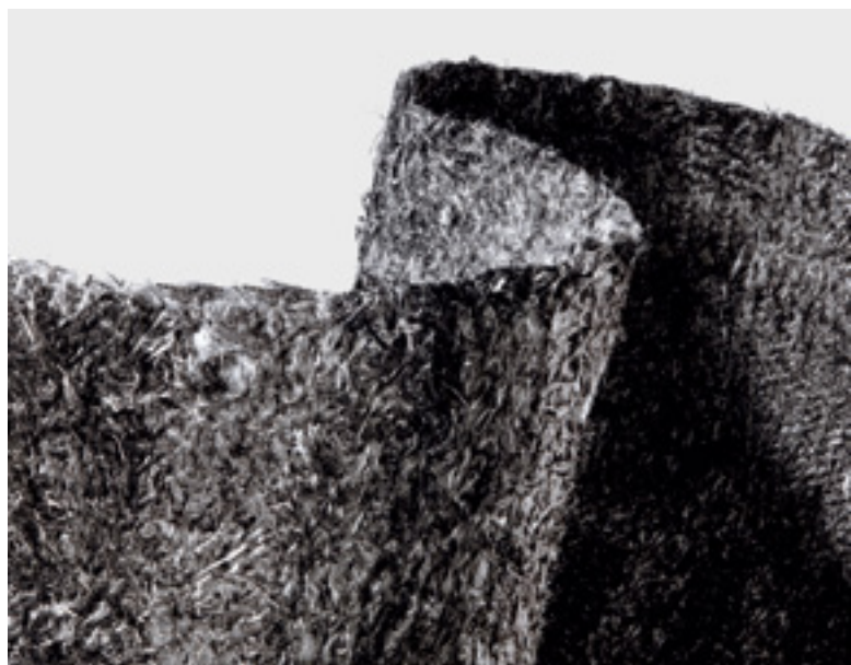
↑ SIGRATEX isotropic non-wovens made from carbon fibers
