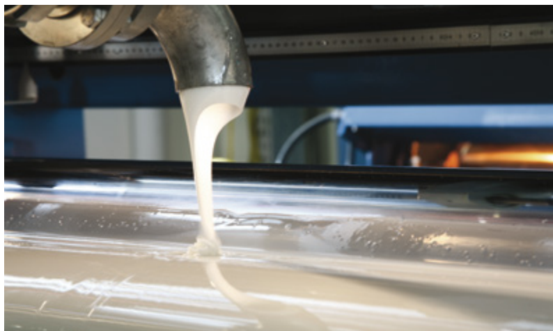
↑ Resin application for impregnation
