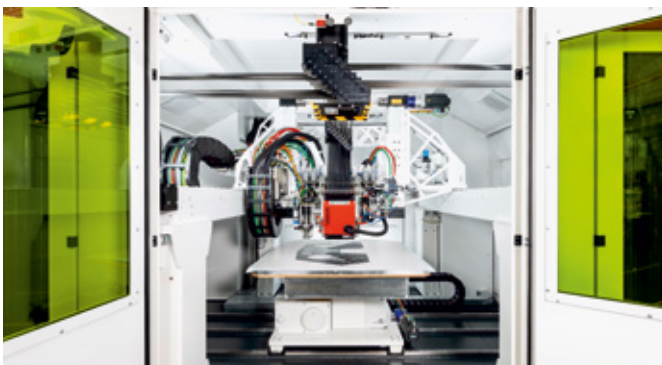
↑ Gantry-based 2D-AFP system for processing TowPreg
