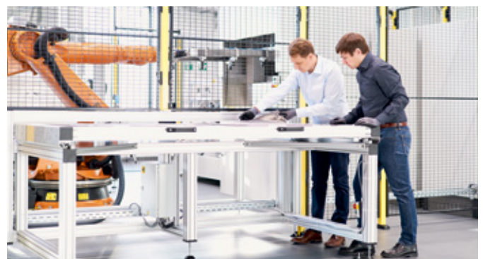
↑ Inserting textile pre-cuts into wet compression molding cell for resin application
