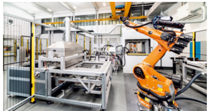
↑ Thermoforming cell with infrared heating field and handling robot
