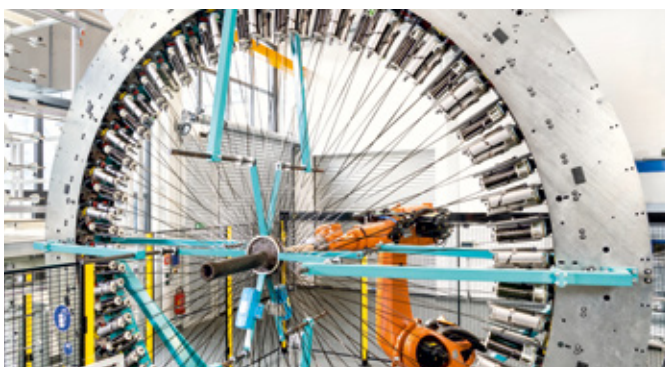
↑ Radial braiding machine with 128 bobbins and handling robot for manufacturing three-dimensional hollow profiles
