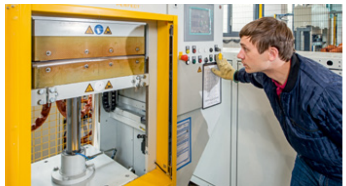
↑ Hot-press for curing prepreg components
