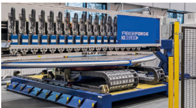
↑ 2D lay-up station for thermoplastic tapes up to 100 mm width
