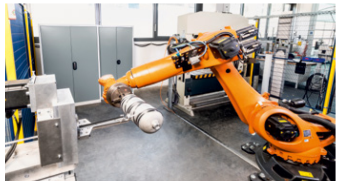
↑ Multifunctional robot winding cell for 3D placement of TowPregs
